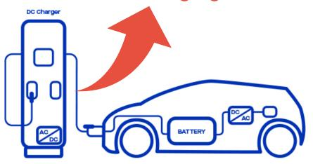
Charging cable, between charger and EV, generates power losses due to his own resistance. DCBM integrates the compensation function
