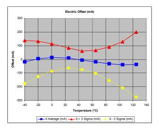
Figure 4-1 : Electric Offset Variation in Temperaturture
