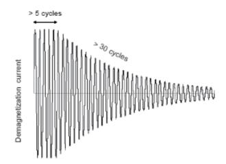
Figure 4-2: Degauss Cycle Current
