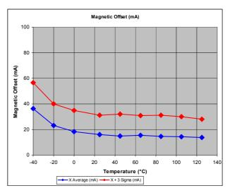
Figure 4-3 : Magnetic Offset Variation in Temperatature
