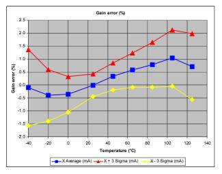
Figure 4-4 : Gain Error Variation in Temperature
