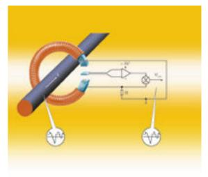
Figure 3-2: Closed-loop Hall Effect Principle
