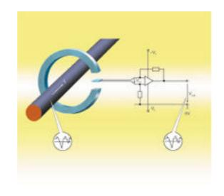
Figure 3-1: Open-Loop Hall-Effect Principle
