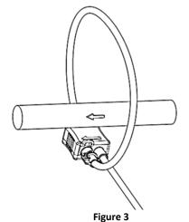
Connect the secondary cable of the ART Rogowski coil to the input terminals of your electronics.
