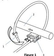
Arrow indicating current direction must be inside the loop (3) when closed.
