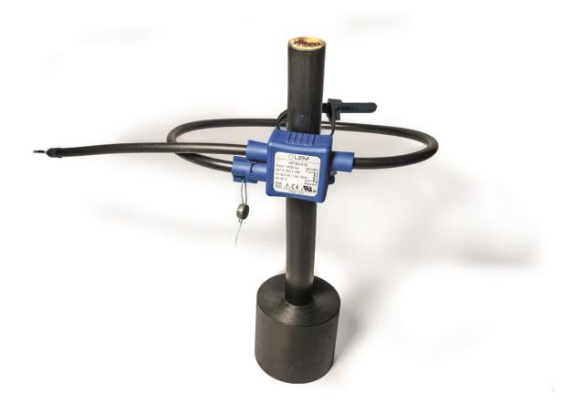
Fig. 8: ART mechanical features: Twist-and-click closure, security seal, and slot to attach the loop to the primary cable.
